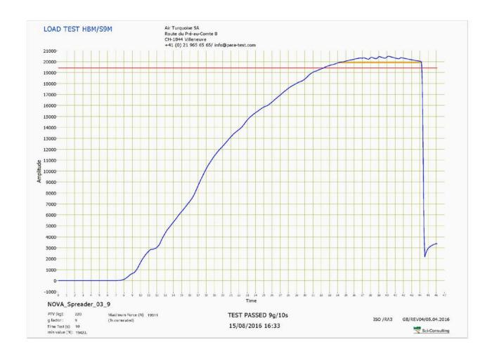
Tested successfully, up to 19711 [N] more during 10 seconds
