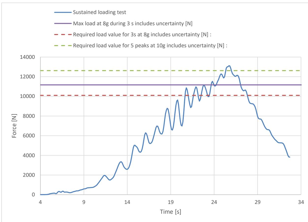
**Sustained loading test results <sup>(3)</sup>**
