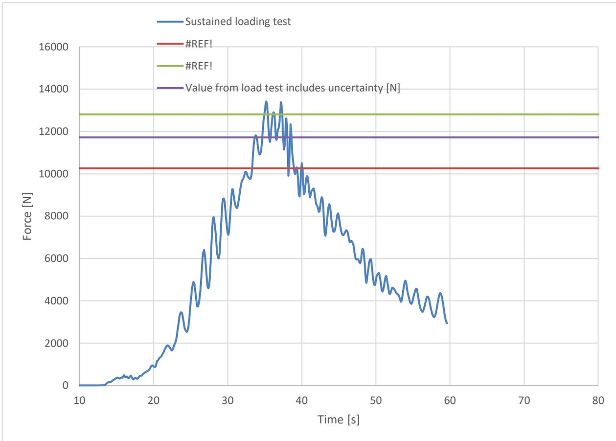
**Sustained loading test results <sup>(3)</sup>**
