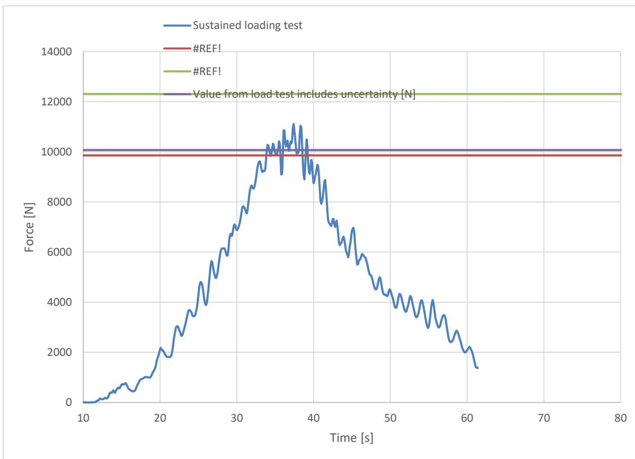
**Sustained loading test results <sup>(3)</sup>**
